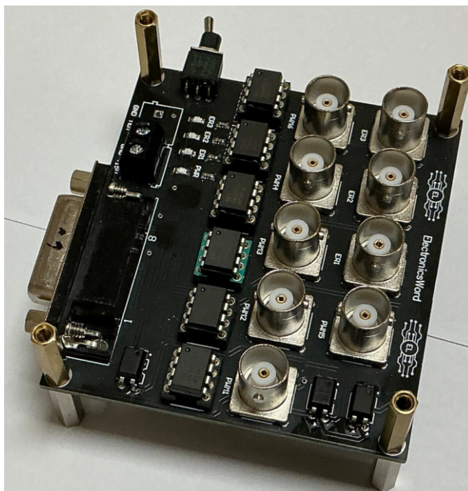
Figure 1: PWM Level Converter module overview
